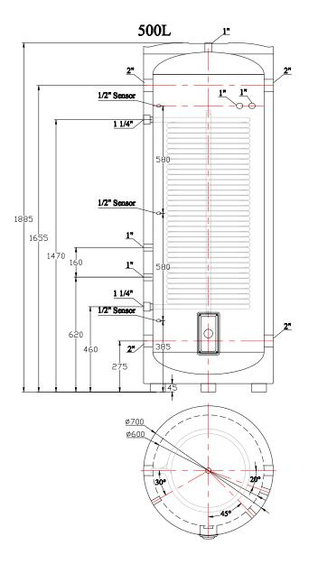
Cylinder Material 304 Stainless Steel Casing Colorbond .5mm Working Pressure 0.6 Mpa Insulation 50mm Polyurethane PTR Relief Valve 700 Kpa Max Inlet Pressure 500 Kpa
